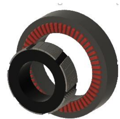
Baseline Design – Conventional north-south pole rotor configuration
