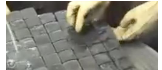
Magnet blocks during manufacturing
