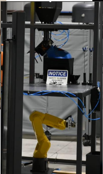
E3 Automated Tube filling in inert environment Partially funded by U.S. Department of Defense / Defense Logistics Agency
